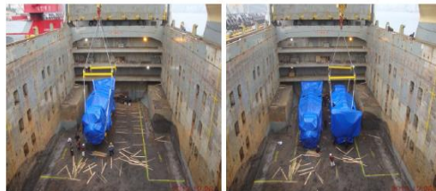
VIEWS OF MAIN ENGINE UNDER LOADING IN AFT SECTION IN NO. 2 LOWER HOLD.
